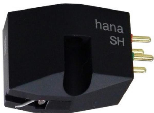
and play back frequencies up to 45kHz – more than twice the highest goal frequency attained with the elliptical styli. The very fine corrugations in the groove required for 45kHz were more easily worn away and so a design was required that could 1) track much higher frequencies and 2) Reduce wear on the record. The first stylus that achieved this was the now famous “Shibata” (named after its inventor).
