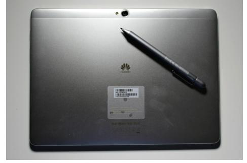
The Huawei MediaPad M2 10.0's dimensions are 239.8 x 172.75 x 7.35mm, and it weighs 490g. The iPad Air 2 that this tablet draws so much inspiration from is 437g.
