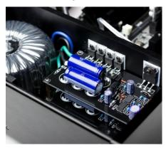
The Host is the first digital music server of CLones Audio and comes equipped with a high performance USB digital audio output, Ethernet port, solid-state drive for music storage and full linear power supply with the super low noise regulator modules.
