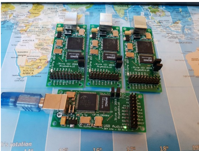
USB => I2S converter using CM6631A:
